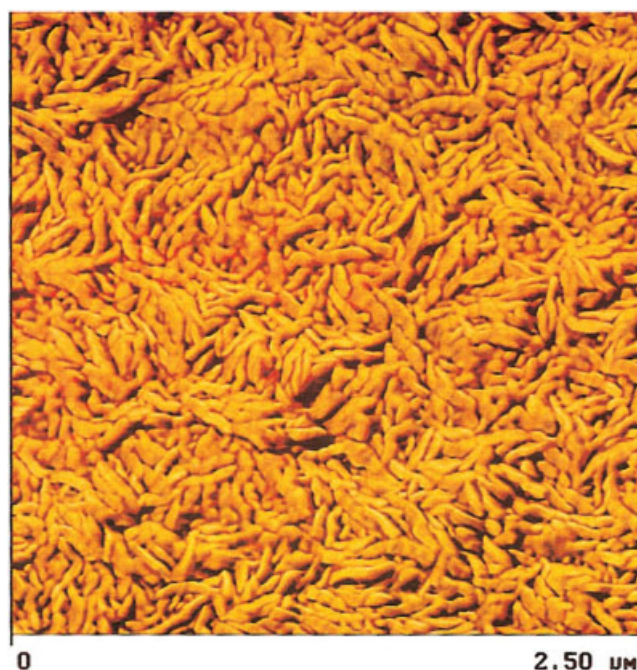
Figure 1 AFM phase image of FEP free-melted surface.
